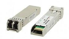
OSP-MM1 is a fiber optic transceiver for 850nm multimode signals. This standard pluggable SFP+ optical module has two LC connectors for reception and transmission of signals over two strands of multimode optical fiber
